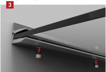
Fit the edge protection rubber onto the glass and then insert the glass into the aluminium profile.
