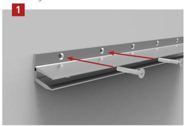
Align the glass panel and secure it with glass fixings.
